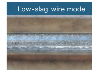
Good weld bead with no defects
